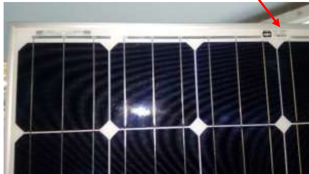
RFID Tag position outside the laminate
